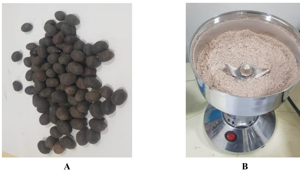
Figure 1. Processing of Nelumbo nucifera (Lotus) seeds. (A) Whole unprocessed dark lotus seeds. (B) Seeds with a homogenous, fine powder using an electrical grinder to facilitate an efficient solvent extraction
